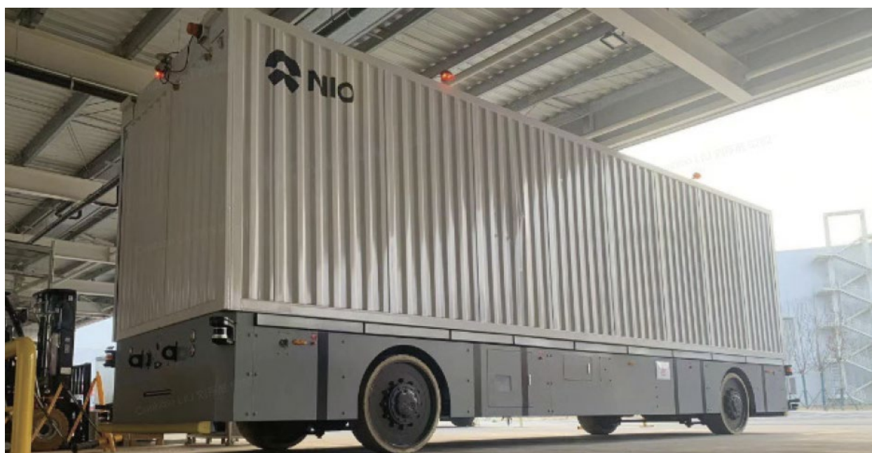
Figure 4: NIO's Unmanned Smart Automated Guided Vehicle (AGV)
